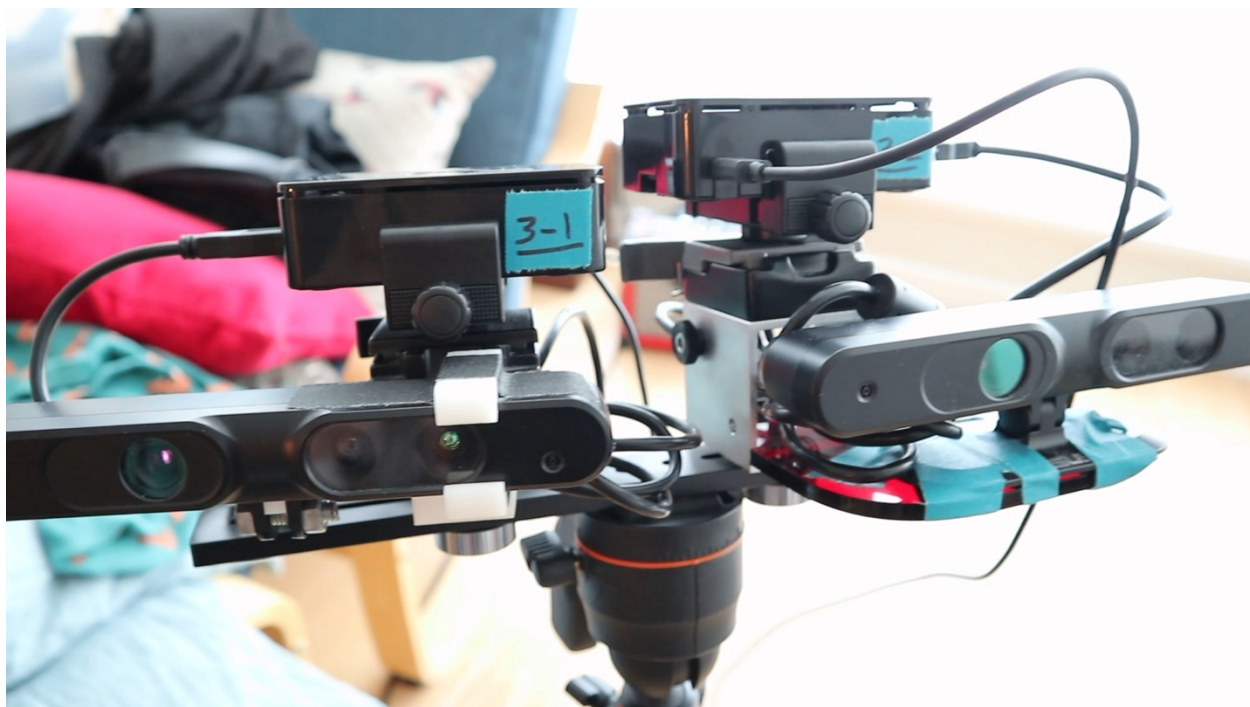
Fig. 7. Asus Xtion cameras (Kinect 1 clones), driven by openFrameworks apps on Raspberry Pis.
