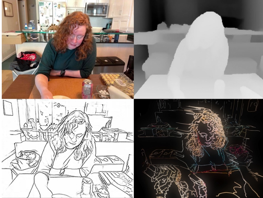
Fig. 26. The stages of the latk_ml_004 pipeline, from top left: RGB input, depth map input, ML system output, and final projection from camera.
